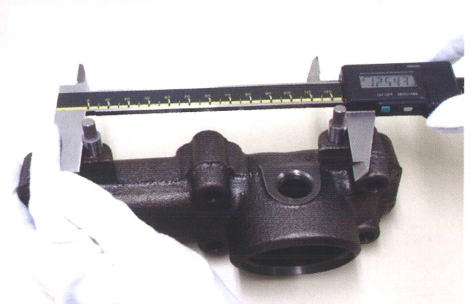
ノギスでねじ穴のピッチを測定 Center-to-center measurement with calipers
